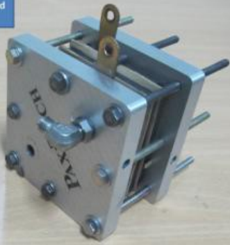
Paxi-Tech 25cm 3 Fuel cell test fixture assembled with two cells.
